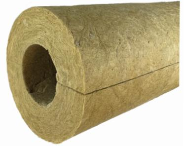
**IFT 1200 Pipe™** is a mandrel wound mineral fibre insulation made from inorganic fibres, designed for steam and process mechanical piping systems operating at temperatures up to 1200°F (650°C). **IFT 1200 Pipe™** provides superior thermal, acoustical and personal protection. This high quality mineral wool insulation is non-wicking, provides high water repellent characteristics and is non-combustable.
